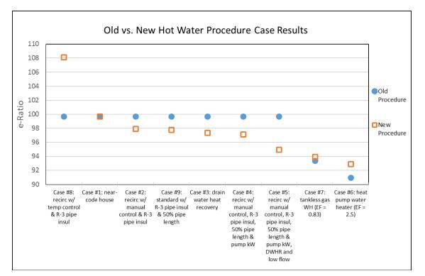
Figure 4. Total e-Ratios predicted by current (old) and proposed (new) DHW calculation procedures for the nine hot water distribution design and equipment efficiency variation cases analyzed, organized from left to right by proposed procedure new e-Ratio.
